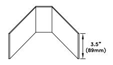
16g ASTM A653 SS Grade 50 Class 1 G60 Bare metal thickness = 0.0538" (1.37mm)
